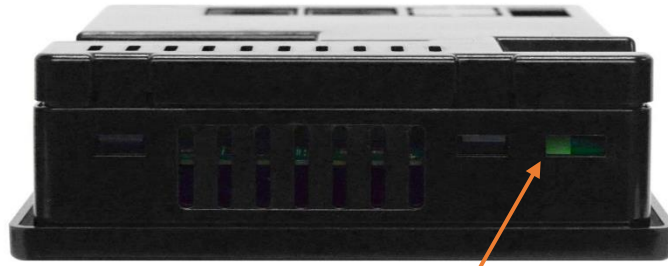
Figure 3.1 – X2 OCS with Mounting Clip Locations
