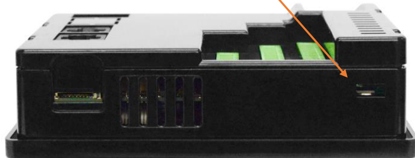
Figure 3.1 – X2 OCS with Mounting Clip Locations
